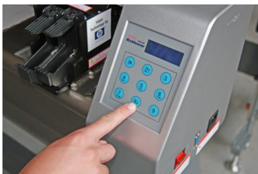
Step three: Press the number key adjust the best printing paper height
